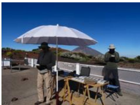
Figure 8: Calitoo absolute calibration setup, Izana observatory, 2018 (Picture credits, F. Bouchard)
